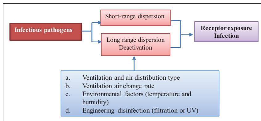
**Figure 4.** Airborne infection pathways and engineering controls.
